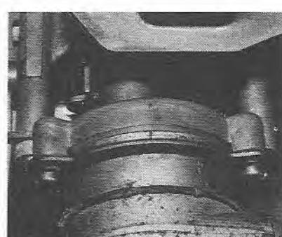
8.66 Automatic choke alignment marks (DFAV type)
