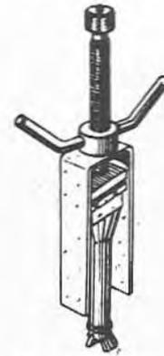
Fig. 6.8 Choke removing tool (Sec 5)
