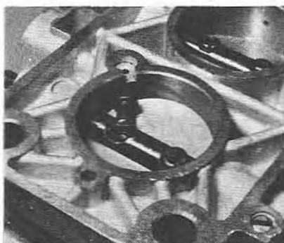
5.52 Removing the secondary throttle valve retaining screws
