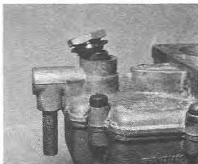
5.2a Removing the filter inspection plug
