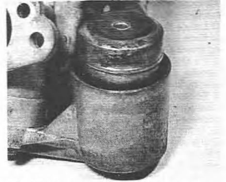
6.15 Lifting the float from the float chamber
