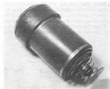
5.6B Solenoid and spring-tensioned disc valve
