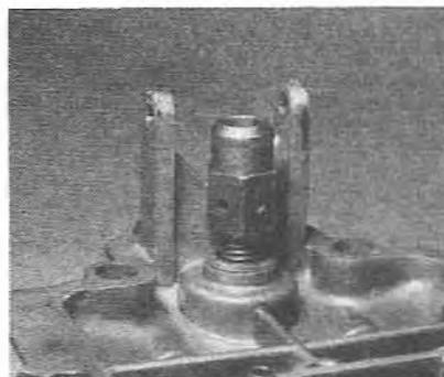
5.9 Removing the needle valve seat (DFAV type)
