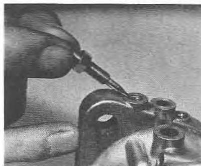
5.28 Removing an air bypass screw
