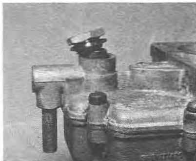
5.2a Removing the filter inspection plug
