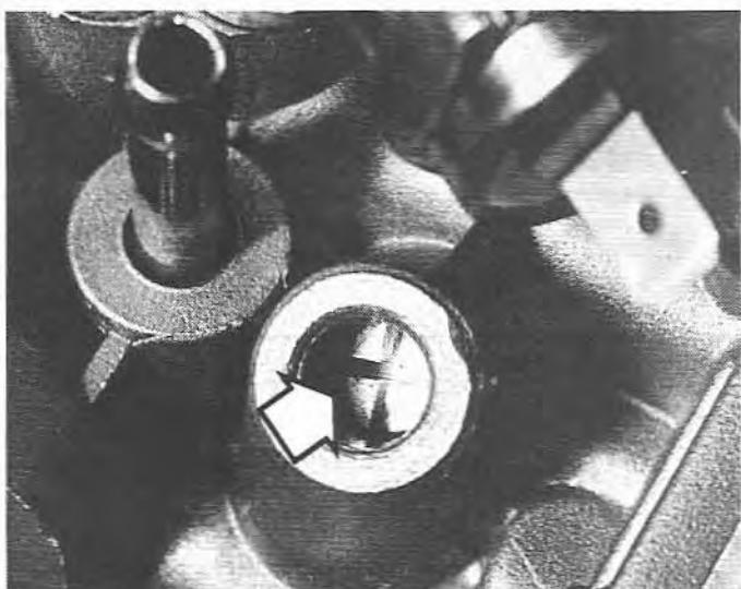
14.8A Mixture adjusting screw location (arrowed)
