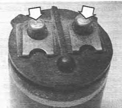
5.10B Solenoid terminals (arrowed)
