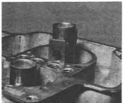
5.32a Removing an auxiliary venturi
