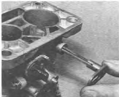
5.42 Withdrawing the secondary shaft from the carburetor body
