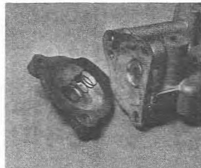
5.35 Removing the diaphragm cover (DFAV type)
