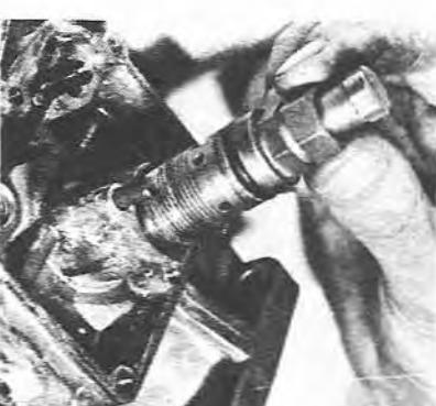
10.6/8 We assembled the jet complete before the float chamber cover.
