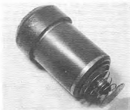
5.6B Solenoid and spring-tensioned disc valve
