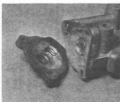
5.35 Removing the diaphragm cover (DFAV type)
