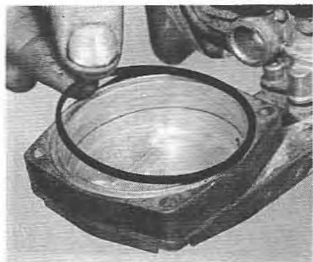
11.14A Removing the upper O-ring ...
