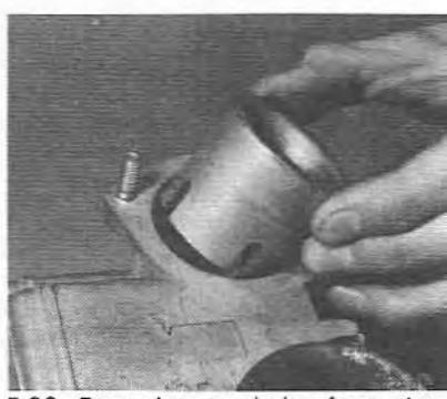
5.38 Removing a choke from the carburetor barrel
