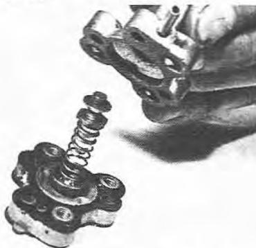
6.11a Note the strength of the spring once the cover is being removed
