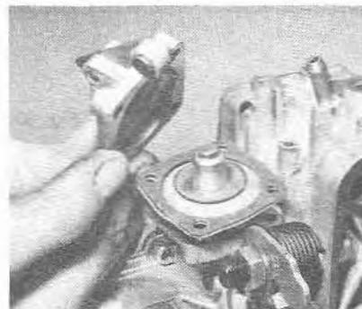
5.24a Removing the accelerator pump cover ...
