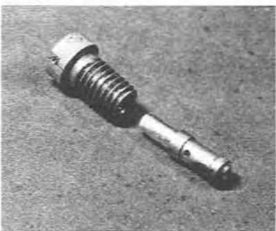
6.15b An idling jet and holder (triple choke type)
