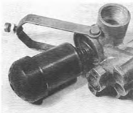
5.6A Removing the solenoid
