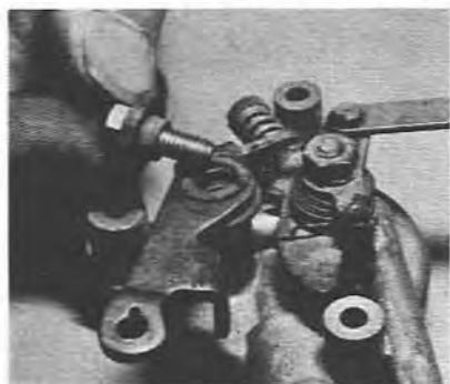
6.30 Removing the fast idle lever (DGAS type)
