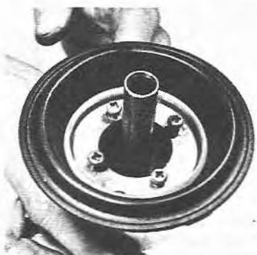
10.12b Tighten the four screws progressively
