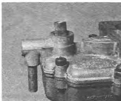
5.2b Removing the fuel filter
