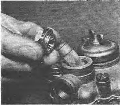
5.2 Removing the fuel filter
