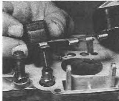
5.4b Removing the float and needle valve
