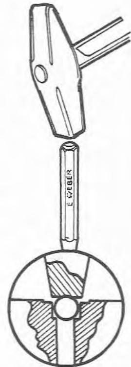
Fig. 6.14 Method of inserting the lead plugs (Sec 6)
