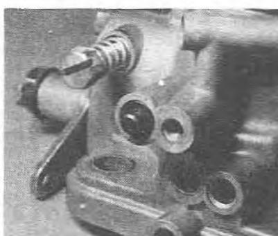
5.29 Automatic choke O-ring seal location (DFAV type)
