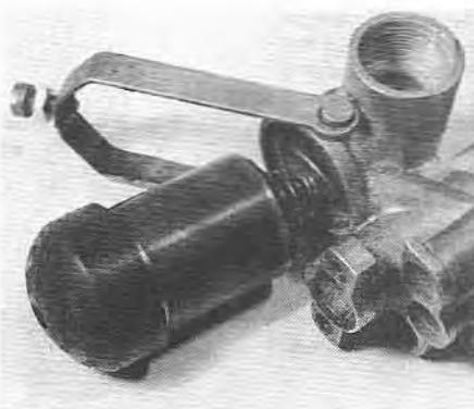
5.6A Removing the solenoid
