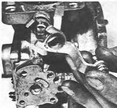
9.5a Main assembly: For clarity other parts of the carburetor body are missing
