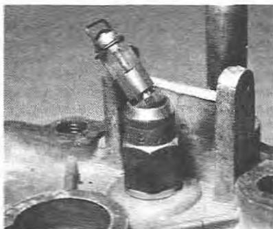
5.7 Removing the needle from the needle valve
