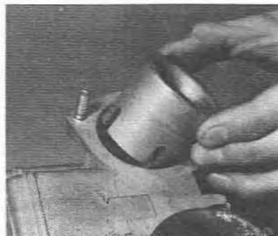
5.38 Removing a choke from the carburetor barrel
