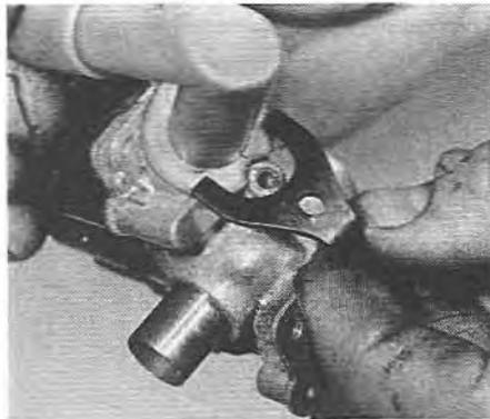
11.19A Air inlet stub and clamp removal
