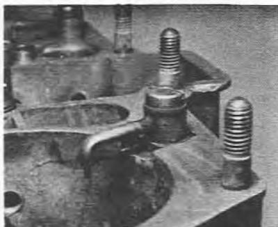
5.15a Location of the accelerator pump delivery valve(twin choke type)
