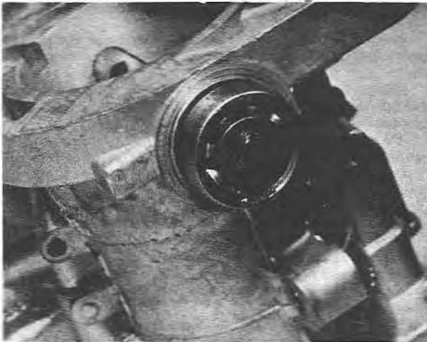
7.9 Fitting the throttle spindle bearing
