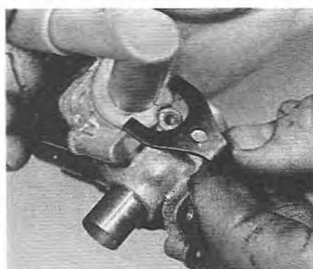
11.19A Air inlet stub and clamp removal
