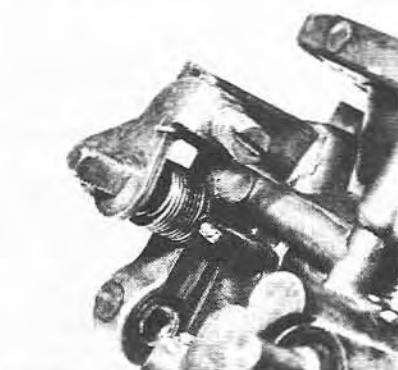
10.10 Note how the spring has been clipped over
