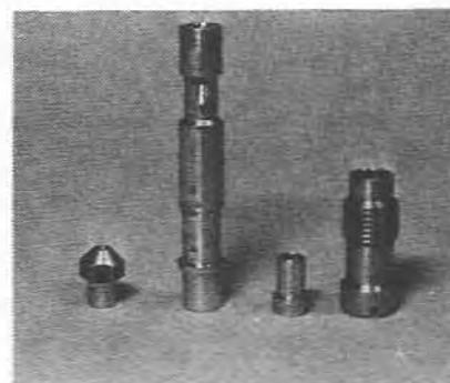
5.15 Component parts of the emulsion tube assembly
