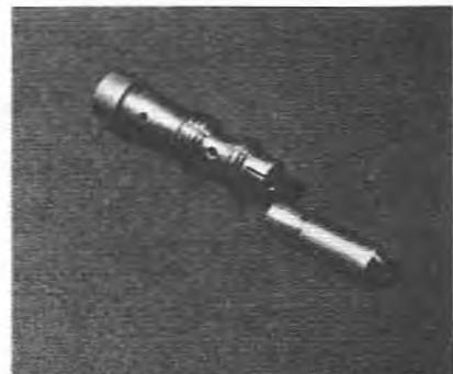
5.14b The idling jet and holder (twin choke type)
