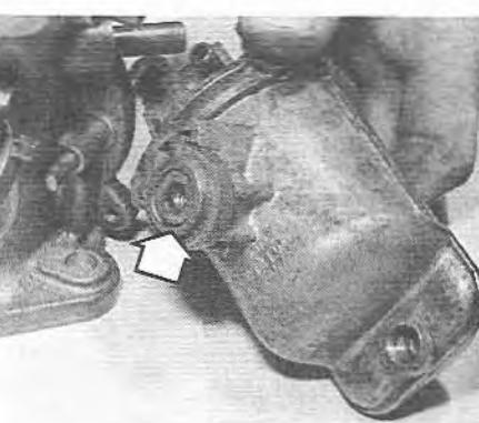
7.11B Float chamber adapter bush location (arrowed)
