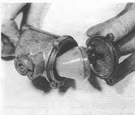
7.16 Removing the float chamber lid
