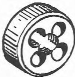
Fig. 4.4 Typical thread die
